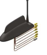
Part number 7000-308 also known as the 'Mallard' is an OEM sleek styled compact sharkfin antenna that can support up to 8 functions. Its robust exterior houses 2x Ultra Wideband antenna elements supporting 700MHz to 6GHz with a minimum 4dBi gain across the whole band\*.
